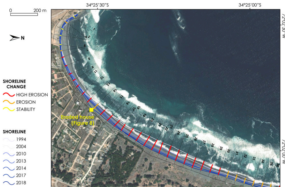
Figure 2. Example of application of the Digital Shoreline Analysis System (DSAS) in Pichilemu. The annual shoreline rate of change is classified according to Rangel-Buitrago et al. (2015) categories: high erosion ( >-1.5 m/yr), erosion (between -0.2 and -1.5 m/yr), stability (between -0.2 and +0.2 m/yr) and accretion ( >+0.2 m/yr). For interpretation of the references to colours in this figure legend, refer to the online version of this article.
